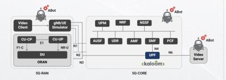
ABot simulated gNB + UE, 5G control plane NF, the video server and the video client in collaboration with Kaloom UPF, executed the test cases, and analyzed the test results and provided video statistic insights/KPIs in a dashboard format.
